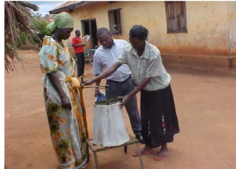
Zabina & Fatuma demonstrating to a CEEWA field staff how a groundnut Huller donated by ICRC to CEEWA beneficiaries in Bulamagi sub county works
